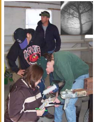
Here a retinal scan camera is being used to take a picture of the illuminated vascular pattern in a lamb's eye. Inset is one of the pictures.
